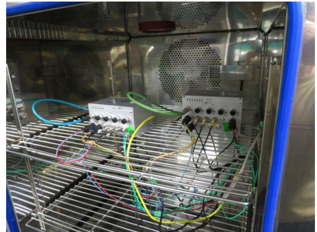
Arrangement of the device under test in the climatic chamber
